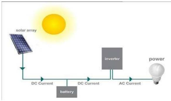
Figure 4.1: Solar PV system
